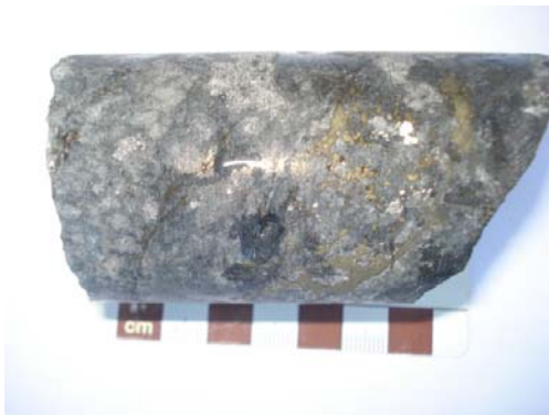
Touro Nickel Project - sulphide mineralised drill core from the current drilling programme.
