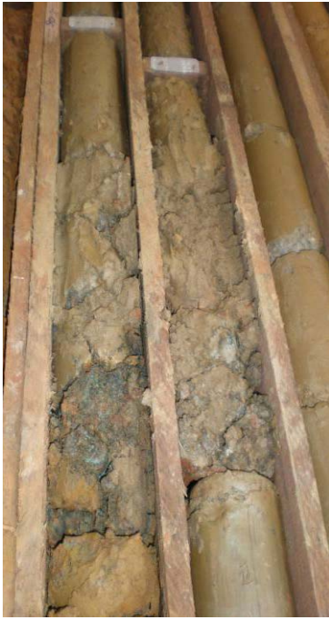
Copper bearing saprolite in drill core recovered from current core drilling programme
