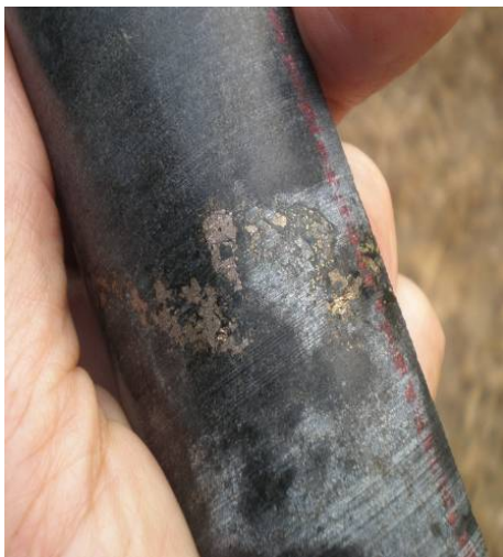
Sulphide mineralised drill core from drill hole TSD-01 which intersected 130m at 0.09% nickel.
