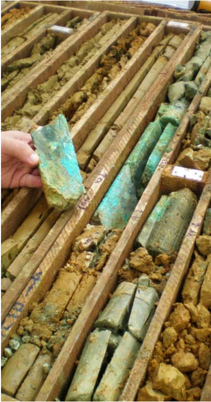
Diamond drill core from previous drilling at Antas South High Grade Copper Deposit
