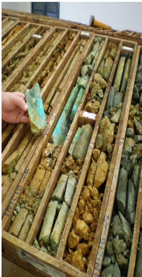
High grade drill core from Antas South Deposit where the visible copper oxide mineralisation is associated with saprolite host rock
