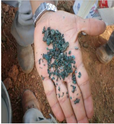
Visible High Grade Copper Oxide mineralisation in drill Chips. High grade zones include 38m at 7.5% Cu from surface
