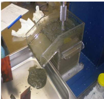
Avanco used the application of sulphidised flotation to recover the Antas South copper oxides
