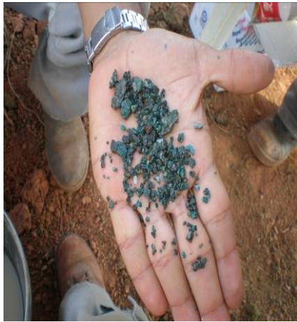
Copper mineralisation in RC drill chips from Antas South.
