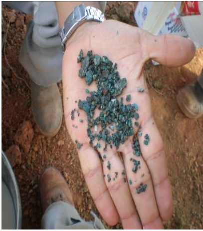
Copper mineralisation in RC drill chips from Antas South.
