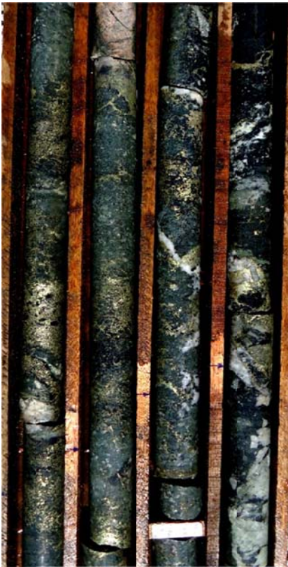
Antas North AAND-13 Matrix 7 and disseminated sulphides
