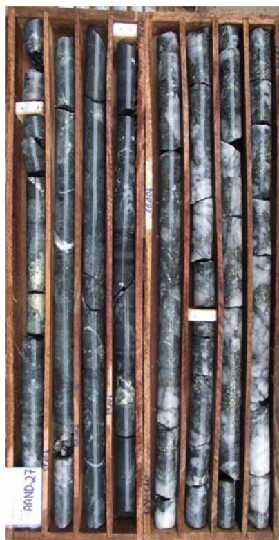
Antas North AAND-27 Disseminated and Matrix 7 sulphides
