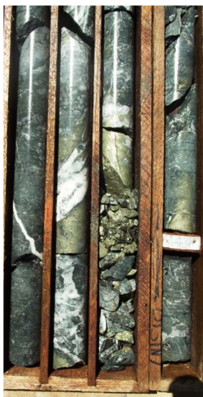
Antas South ARVD-146 Semi- massive and disseminated sulphides
