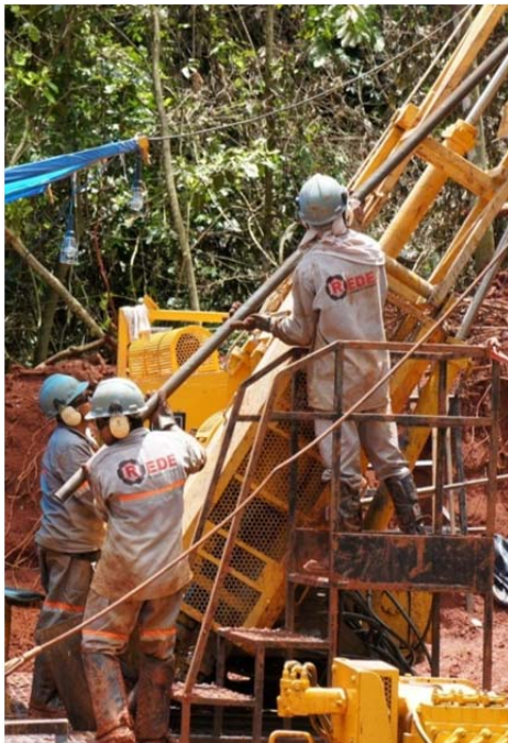
Diamond core drilling of iron ore at the Trindade North Project
